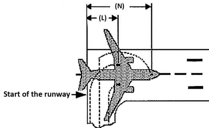
Where the aeroplane manufacturer does not provide the appropriate data, the calculation method given in (b) may be used to determine the alignment distance.
