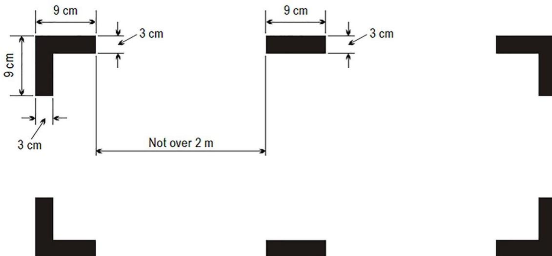
**AMC1 NCO.IDE.A.165 MARKING OF BREAK-IN POINTS****MARKINGS — COLOUR AND CORNERS**
