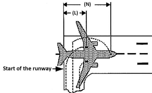
Where the aeroplane manufacturer does not provide the appropriate data, the calculation method given in (b) should be used to determine the alignment distance.
