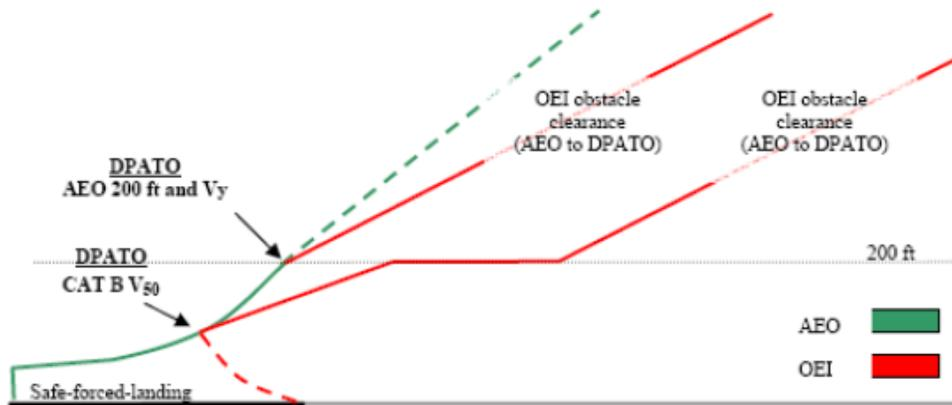
Otherwise, and if scheduled in the AFM, the AEO distance to 50 ft ( $V_{50}$ ) — determined in accordance with CS/JAR 29.63 — can be used (see Figure 7). Where this distance is used, it will be necessary to ensure that the  $V_{50}$  climb out speed is associated with a speed and mass for which OEI climb data are available so that, from  $V_{50}$ , the OEI flight path can be constructed.
