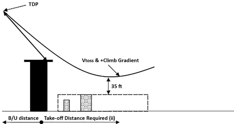
The main difference is that drop down below the level of the take-off surface is permitted. In the drop down phase, the Category A procedure ensures deck-edge clearance but, once clear of the deck-edge, the 35 ft clearance from obstacles relies upon the calculation of drop down. Subparagraph (b) of [AMC1 CAT.POL.H.205\(b\)\(4\)](#) is applied.
